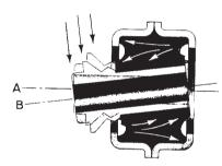
**B.** Displacement of the neoprene, as indicated by arrows, compensates for angular misalignment of the connected shafts.
