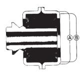
**B.** Position of biscuit after thrust load has been imposed. The flow of the neoprene permits controlled end float. Thrust loading is transmitted smoothly and uniformly. **Torsional deflection resulting from torque loads and torsional vibration A.** Centreline of biscuit before application load \_\_\_\_\_A
