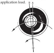
**B.** Imposition of a torque increases pressure in the direction of the load, and reduces pressure in the opposite direction. Because of its initial preloaded condition the neoprene remains under compression throughout its volume at maximum torque load.
