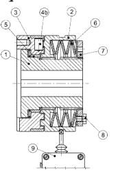
The Synchron clutch functions in much the same way as the Safegard, and has similar construction in except the balls 4a are replaced by seven rollers 4b. The rollers are unequally spaced so the clutch will only engage drive in one angular position, providing full synchronisation of the drive.
