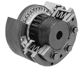
The Safegard CSF Clutch uses a large number of equally spaced balls to provide the drive, and the clutch ratchets from one drive position to the next in the event of an overload. The design allows for high operating speeds, and the possibility to recapture drive in the event of an inertia created overload during starting, but do not provide any synchronisation between input and output.
