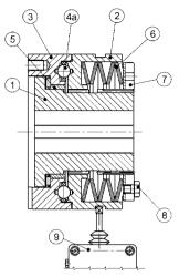
During normal operation the drive is transmitted by the sliding hub 2, which is connected by a spline to the main hub 1, and via a ring of balls 4a to the output flange 3. Drive is maintained by the springs 6 exerting pressure on flange 2, so keeping the balls in their respective indents in flange 2 & 3.
