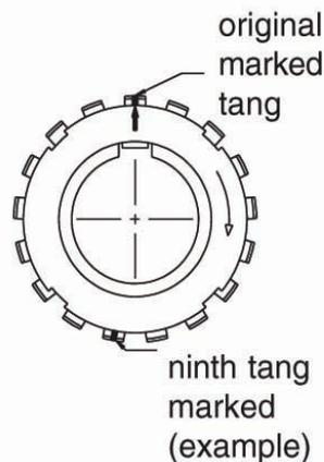
3. Mark a lock washer tang in any suitable manner, and the adjacent, mating area of the lock nut.
