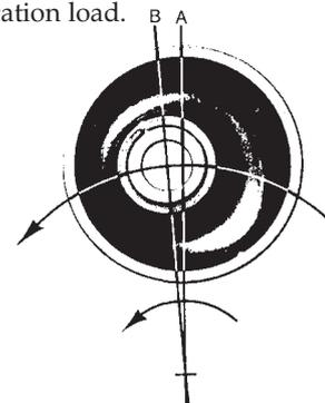
B. Imposition of a torque increases pressure in the direction of the load, and reduces pressure in the opposite direction. Because of its initial preloaded condition the neoprene remains under compression throughout its volume at maximum torque load.
