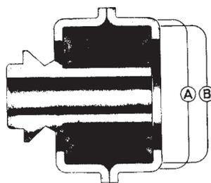
B. Position of biscuit after thrust load has been imposed. The flow of the neoprene permits controlled end float. Thrust loading is transmitted smoothly and uniformly.
