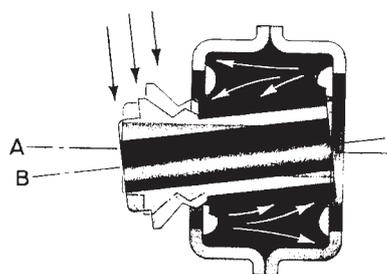
B. Displacement of the neoprene, as indicated by arrows, compensates for angular misalignment of the connected shafts.
